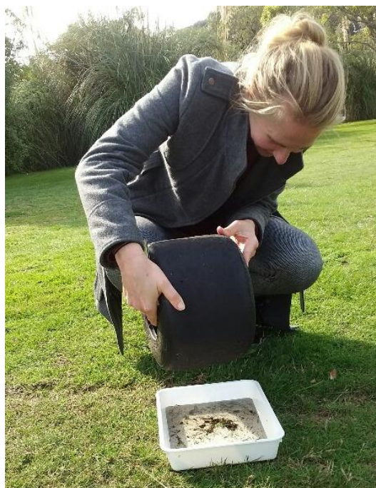
Figure 2) Emptying a tyre trap into a white container.
