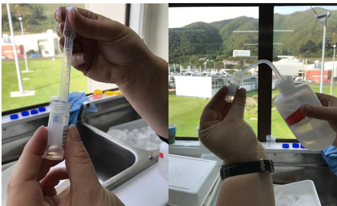
Figure 9a) remove as much water from the tube as possible; b) replacing water with 70% ethanol.
