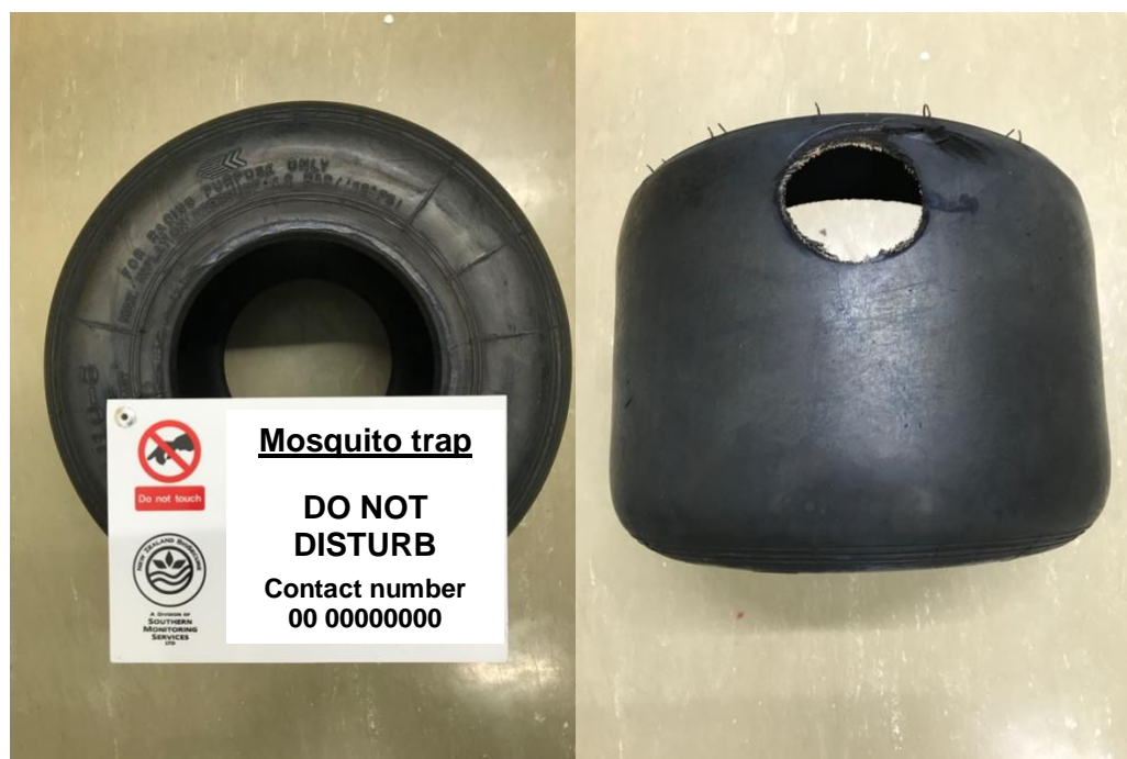
Figure 1a) Tyre trap with signage. b) Hole drilled to empty the content
