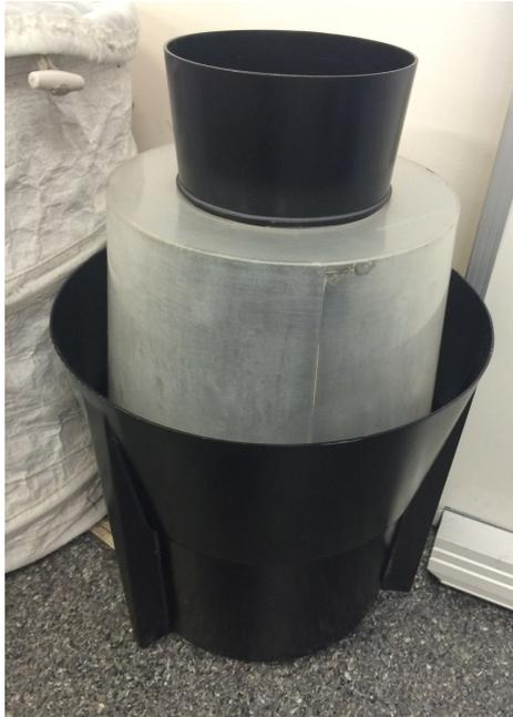
A recently developed novel trap (passive trap) has proven successful in capturing large numbers of *Aedes*, *Anopheles*, *Culex* and *Verrallina* mosquitoes without the use of power. These rely upon luring mosquitoes into a translucent “passive” trap from which those mosquitoes, attracted to the light entering the translucent body, cannot find their way out.
