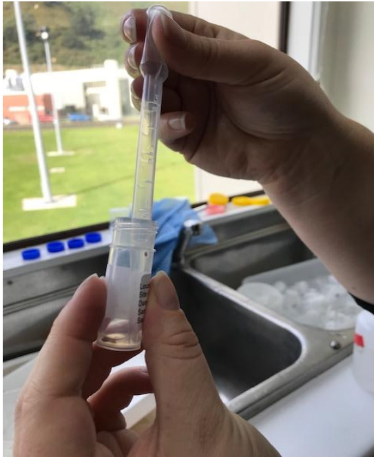
Figure 9a) remove as much water from the tube as possible; b) replacing water with 70% ethanol.
